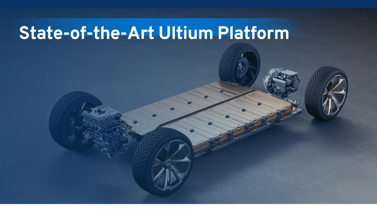
The Ultium platform is a critical element in GM's all-electric future. As a hyperscale platform based upon a core set of modular batteries and drive units, Ultium perfectly embodies the "less is more" concept. The platform also adopts a wireless battery management system, the first of its kind used on a production electric vehicle (EV). It will continuously increase the cost-effectiveness of EVs through scale and technological innovations.
