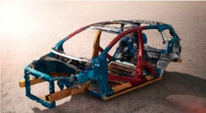
GM is using its third-generation high-strength steel in the new Chevrolet LOVA RV from SAIC-GM. The new steel reduces the weight of selected body components by 20 percent. ( In theory, reducing a vehicle’s body weight by 10 percent increases fuel economy by 6-8 percent. )
