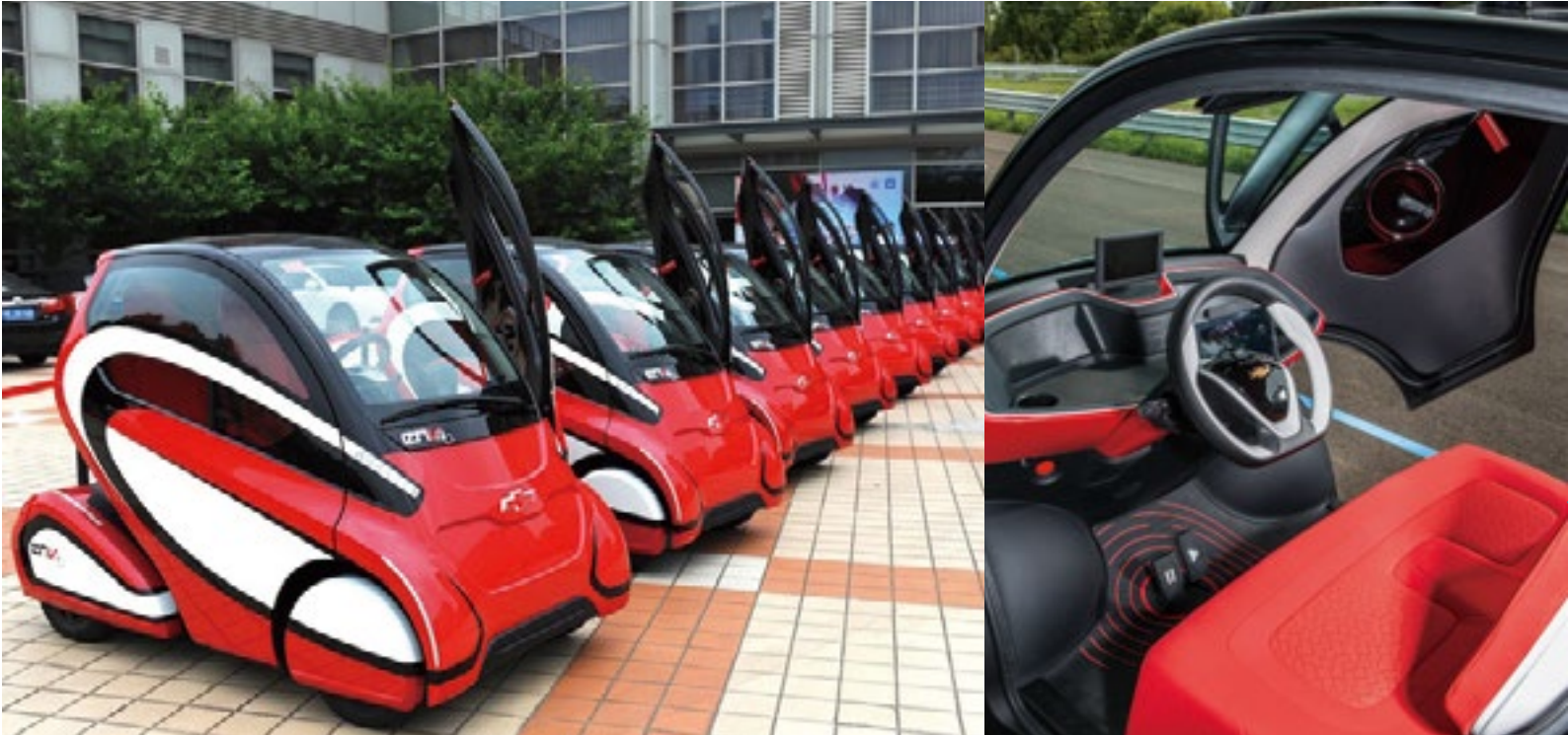
A driver uses a swipe card to enter, pay for and then drive a vehicle. The EN-V 2.0 has a rearview camera, GPS and the OnStar system, and supports tablets and smartphones.
